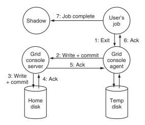
19.13 FIGURE The Grid Console permits more flexible I/O coupling. As the job runs, it writes output data to the agent, which stores it on the temporary disk or forwards it to the server. When the job wishes to exit, it informs the agent, which must then force all output to the server. If successful, the job is informed and may indicate completion to the shadow.
