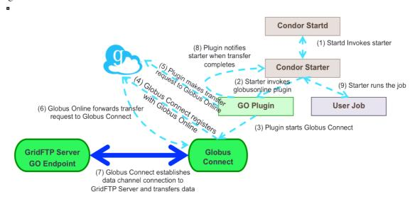
Figure 5: Transferring input files using Globus Online plugin
